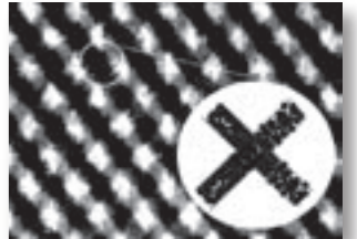
EA Toner uniformity (shape and diameter) reproduces screens precisely, without unwanted toner dispersion.
