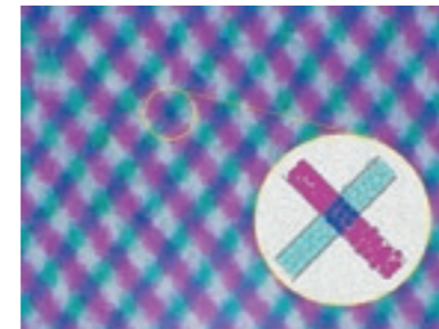
Conventional toner suffers from screen dispersion because of particle size and uneven shape.
