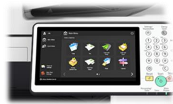
10.1" TFT LCD WSVGA Color Touch-panel
